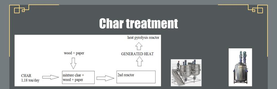
The char  $\rightarrow$  is mixed with woody biomass and wastepaper, the blend produced is used in co-gasification in a second reactor to generate the heat required required by the pyrolysis reactor.
