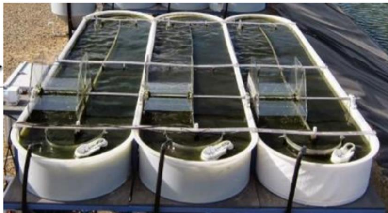
Pilot-Scale Raceways (2-5 day HRT)
